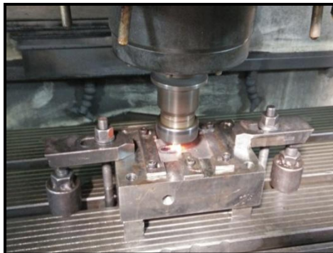
Figure 2: Friction stir processing of SA 210 grade A1 using WC tool on VMC at 1600 rpm.
